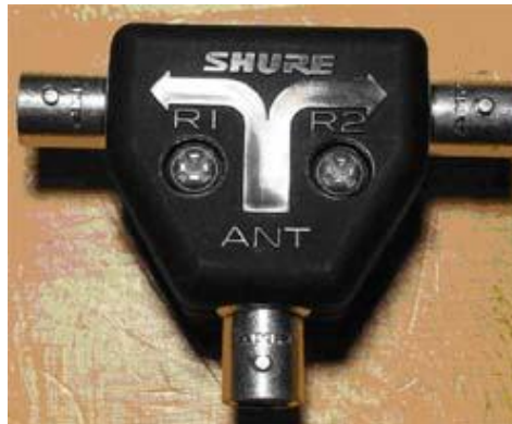
The UA221 passes dc from 'ANT' to R1 but blocks dc from R2
