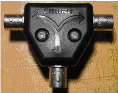
The discontinued UA220 passed dc from the lower BNC to upper BNC's
