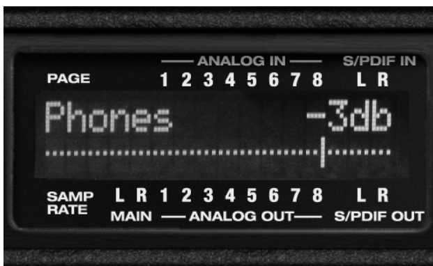
Figure 6-3: For many settings, the LCD “zooms in” on the setting as you adjust it.
