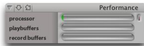
Figure 10-6: When adjusting the buffer size to reduce monitoring latency, watch the 'processor' meter in Digital Performer or AudioDesk's Performance Monitor. If you hear distortion, or if the Performance meter is peaking, try raising the buffer size.
