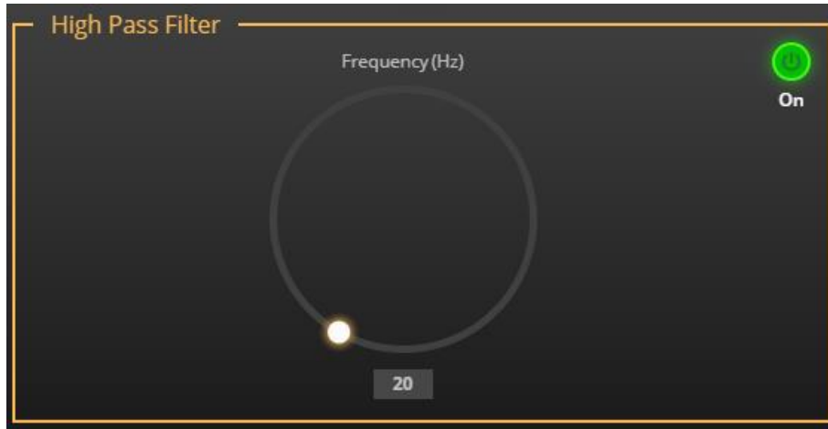
Figure 26: Processing View – HPF Module
