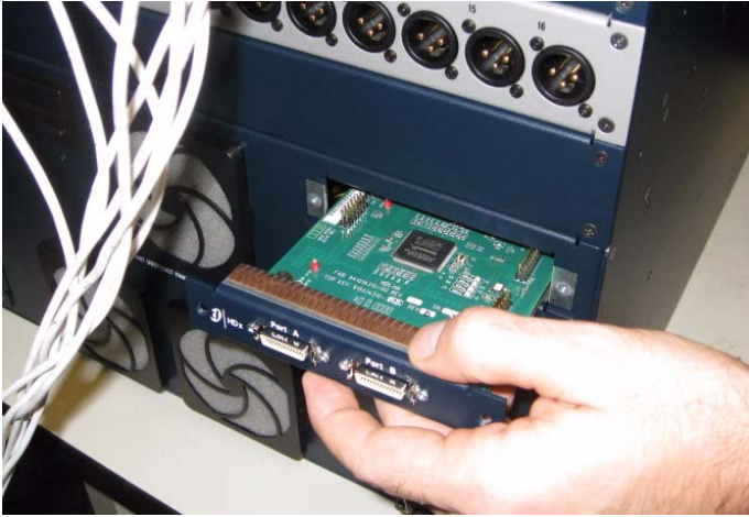
Installing the HDx card in the back of the Mix Rack
