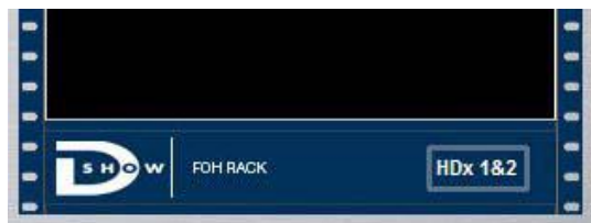
Two HDx cards indicated in the FOH Rack icon in the Devices page
