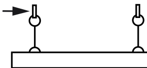
Fig. 16: Cable pick Dual pickpoint operation
