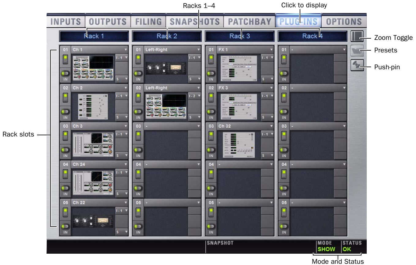
Figure 15. Plug-In racks and rack slots, Main view, with custom rack names shown.
