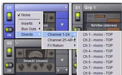
Assigning a channel Direct Out as a plug-in input source in the Plug-Ins page
