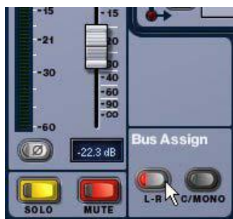
Assigning a Group output to the Main busses from the Output page
