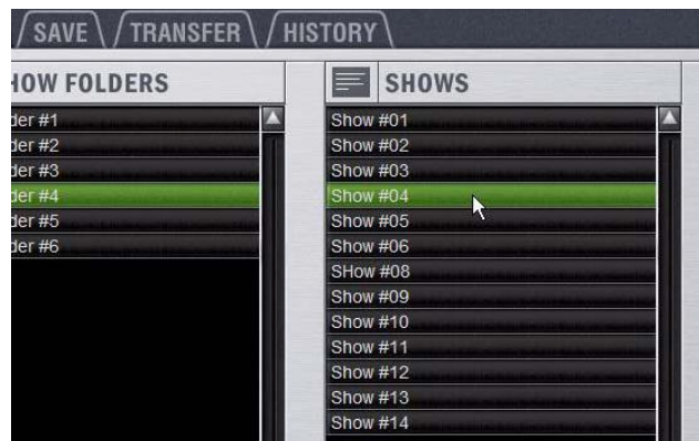
Show Folders and Show files in the Load tab of the Filing Page
