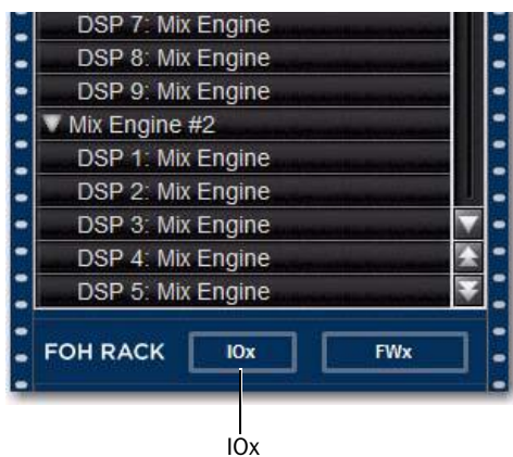
Detail of Devices page indicating presence of an IOx card
