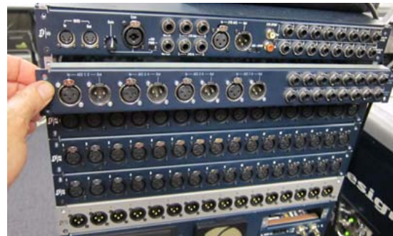
Sliding the IOx card into Slot A
