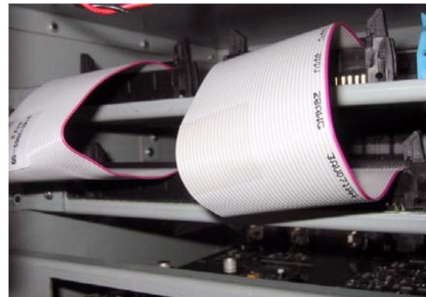
Ribbon cables connecting the IOx card to the IO card
