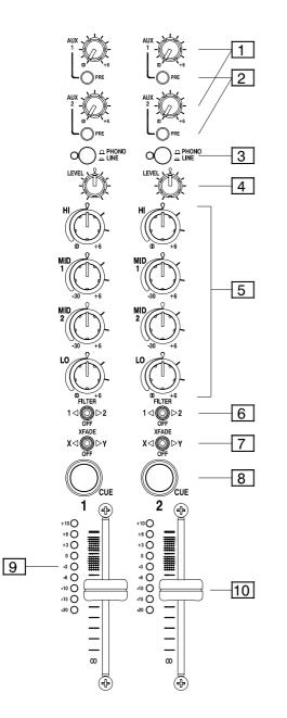
1 AUX 1-2 sends. Adjust the levels of the channel signals to the stereo Aux outputs. Turn fully anticlockwise to turn the signal off, fully clockwise for a maximum +6dB boost.
