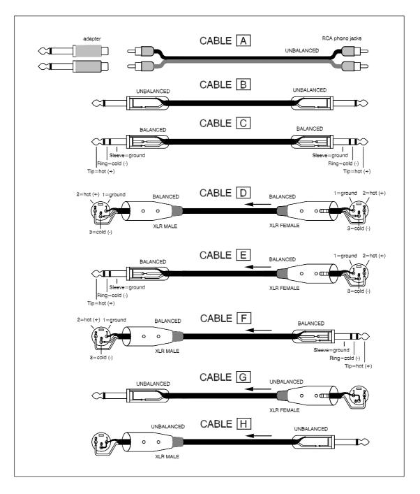
1 **CH1-2 MIC input**. Balanced XLR. Plug in a DJ, guest or announcement microphone here. Use good quality low impedance dynamic mics such as those specifically designed for vocals. Do not use high impedance or unbalanced microphones, or condenser types which require phantom power. Use professional grade balanced cables wired as CABLE D. Use the best cable and connectors you can afford as these are typically subject to intense use and abuse in the club environment.
