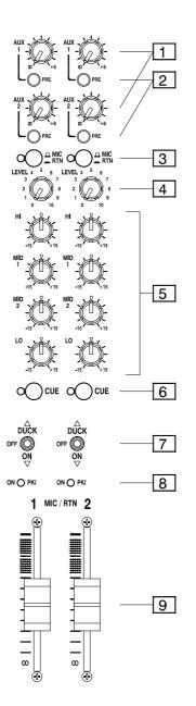
**AUX 1-2 sends**. Adjust the levels of the channel signals to the stereo Aux outputs. Turn fully anticlockwise to turn the signal off, fully clockwise for a maximum +6dB boost.
